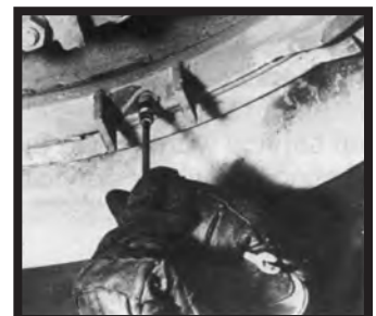
Running wire through the stem of a single piece wheel.
