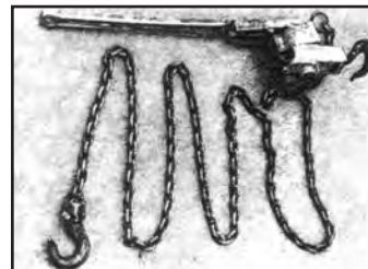
7. Coffin hoist (1/2 ton capacity). This tool expands the bead on tapered bead seats, so that a tubeless tire will take air.
