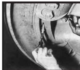
Removing valve core from single piece wheel.
