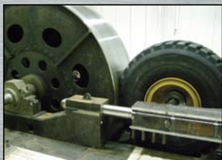
Titan's bull wheel (left), the largest in the world, simulates real world usage on Titan's new 59/80R63 giant tire. The bull wheel is able to apply as much as 500,000 pounds of pressure on a tire, while running at speeds of up to 45 miles per hour. This 63-inch tire is approximately 13.5 feet tall and weighs approximately 12,500 pounds.
