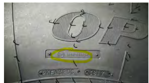
Example of the ECE Marking Note: The location of the marking on the tire may vary
